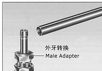
To eliminate the problem, use a male adapter into the female port.
